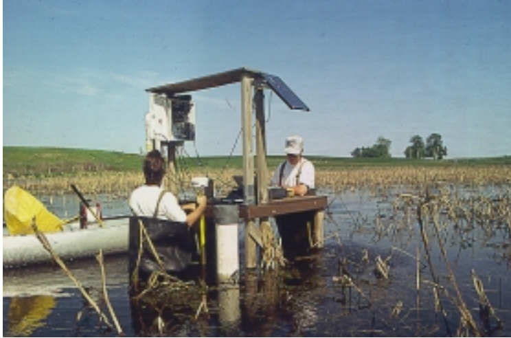
Figure 10. Well platform at site CD 4 within the restoration site. Shown are the data logger enclosure, surface water stilling well and solar panel (photo by Carol Thompson).
