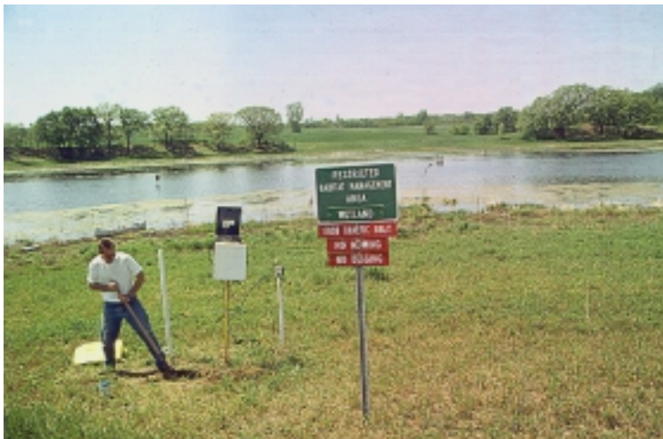
Figure 12. Well site CD 2 within the restoration site. Shown are the data logger enclosure and solar panel with well CD 2B at left and well CD 2A at right (photo by Carol Thompson).
